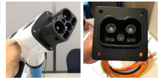
Fig. 27. AC and DC plugs standard in Japan, America, Europe, and China.
