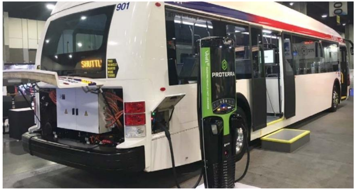
Fig. 37. a plug-based charging station for E-bus (high) and a depot charging station for E-buses (low).
