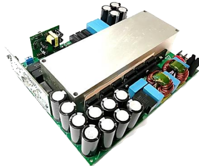
Fig. 10. Conductive AC charger block diagram and a sample.
