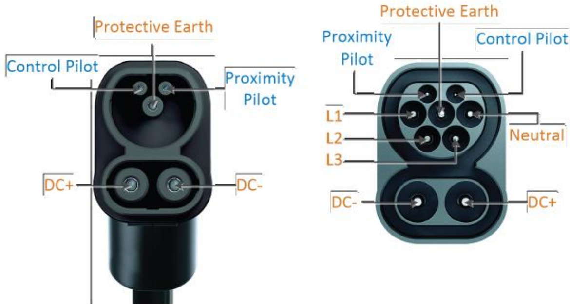
Fig. 29. Pin out of the CCS1 (high) and CCS2 (low) for both plug and socket.
