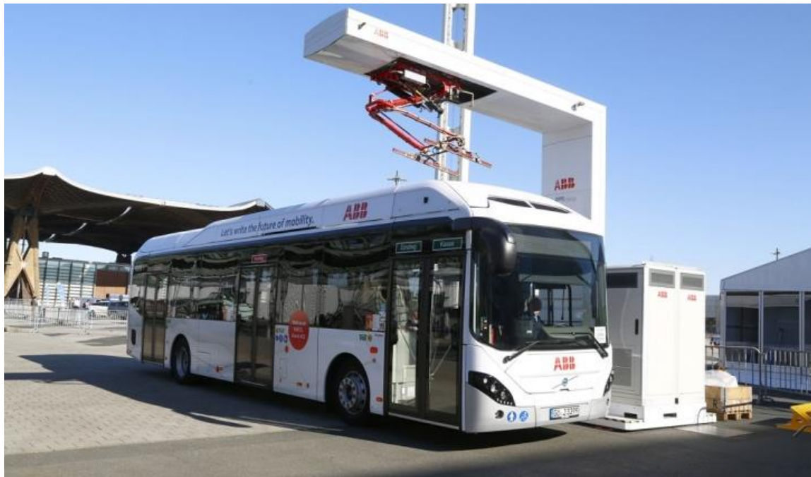
Fig. 38. A flash charging station (high) and an opportunity charging station based on inverted pantograph (low).
