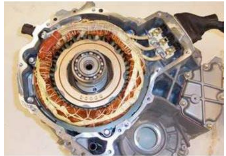
Fig. 19. A BLAC structure: Cross section(left), and a real sample (right).
