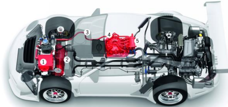
1. Power electronics 2. Portal shaft with two electric motors 3. High-voltage cable 4. Electrical flywheel battery 5. Power electronics
