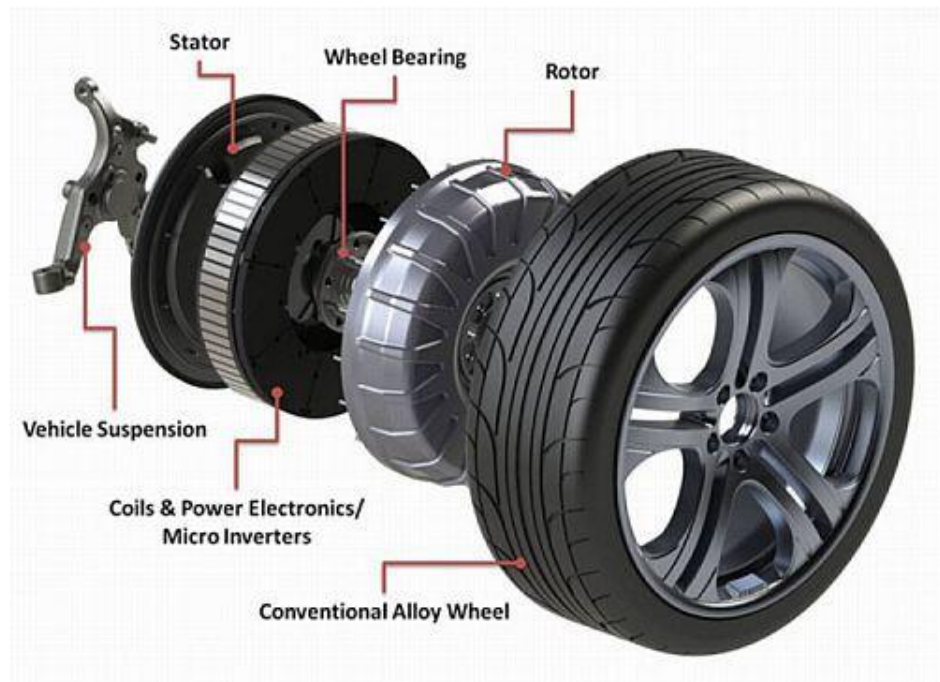
Fig. 51. Mounting of various part in a wheel for in-wheel drive.
