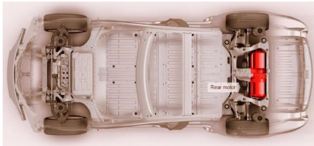
Fig. 49. Two rear wheel drive vehicles: motor, gear, and differential as a single unit (Tesla Model S (left); in-wheel type (Nissan Blade Glider (right))).
